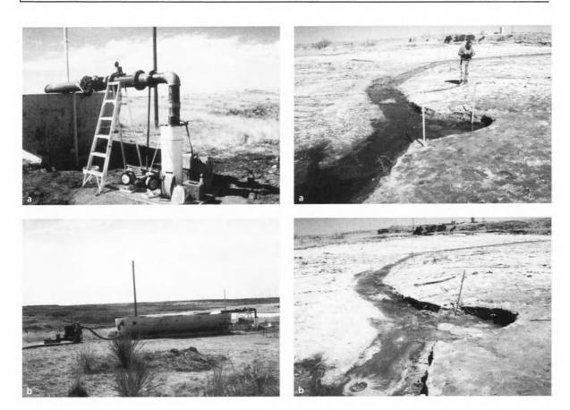
Fig. 5.1. a Childress County, Texas, Jonah Creek, a tributary of Red River. Instrumentation for measurement of water levels and monitoring discharge during pumping test.
